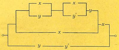
Draw an equivalent circuit as simple as possible. Show that current will flow through the circuit if and only if the switch x is on.
